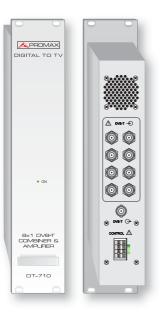
The **DT-710** is a combiner with 8 inputs and an output designed to mix output RF signals of **COFDM** modulators and transmodulators with DTT channels available in the area. The system provides an amplified output of 114 dB $\mu$ V (+6 dBm) frequently required in **SMATV** systems. This is a solution of higher quality than those that often use Z connections, given that preserves better the original quality and maintains lower noise levels.
