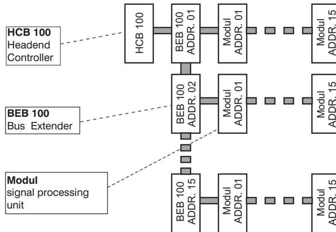
**The number of the possible module connections (00 ... 15) to a BEB 100 depends on the total power consumption of this line!**
