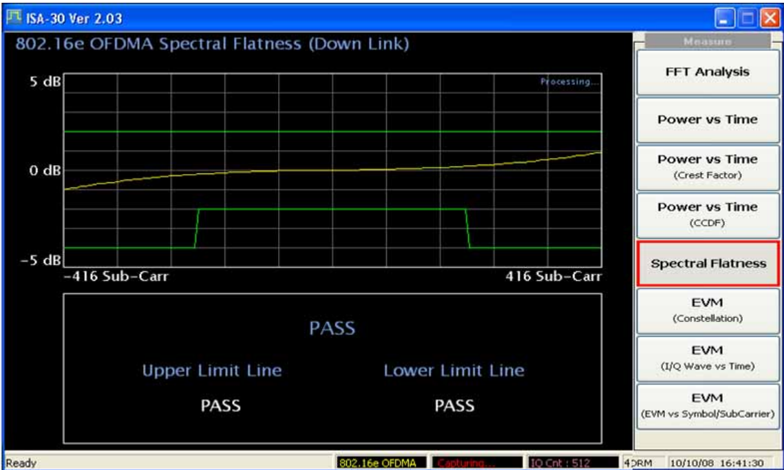
Fig. 2-18 Spectral Flatness Measurement (802.16e DL signal)
