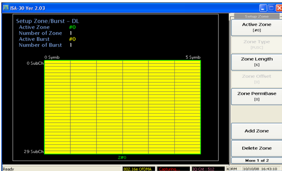
Fig. 2-20 Set parameters for zone (802.16e DL signal)
