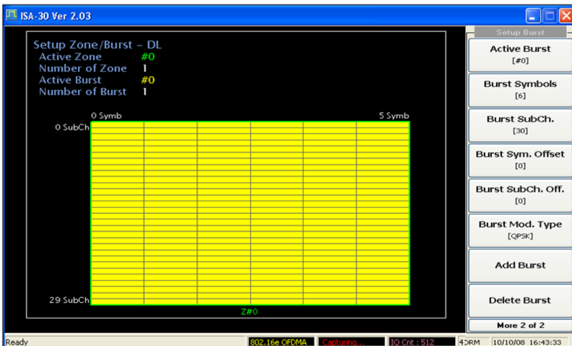
Fig. 2-21 Set parameters for Burst (802.16e DL signal)
