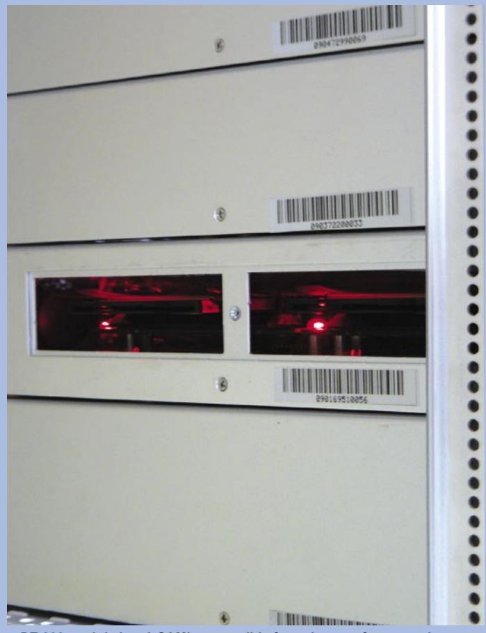
■ DT-302 module has 2 CAM's accessible from the top after removing a cover. They are capable to decipher scrambled channels. Of course, you need to put in valid smart cards.
