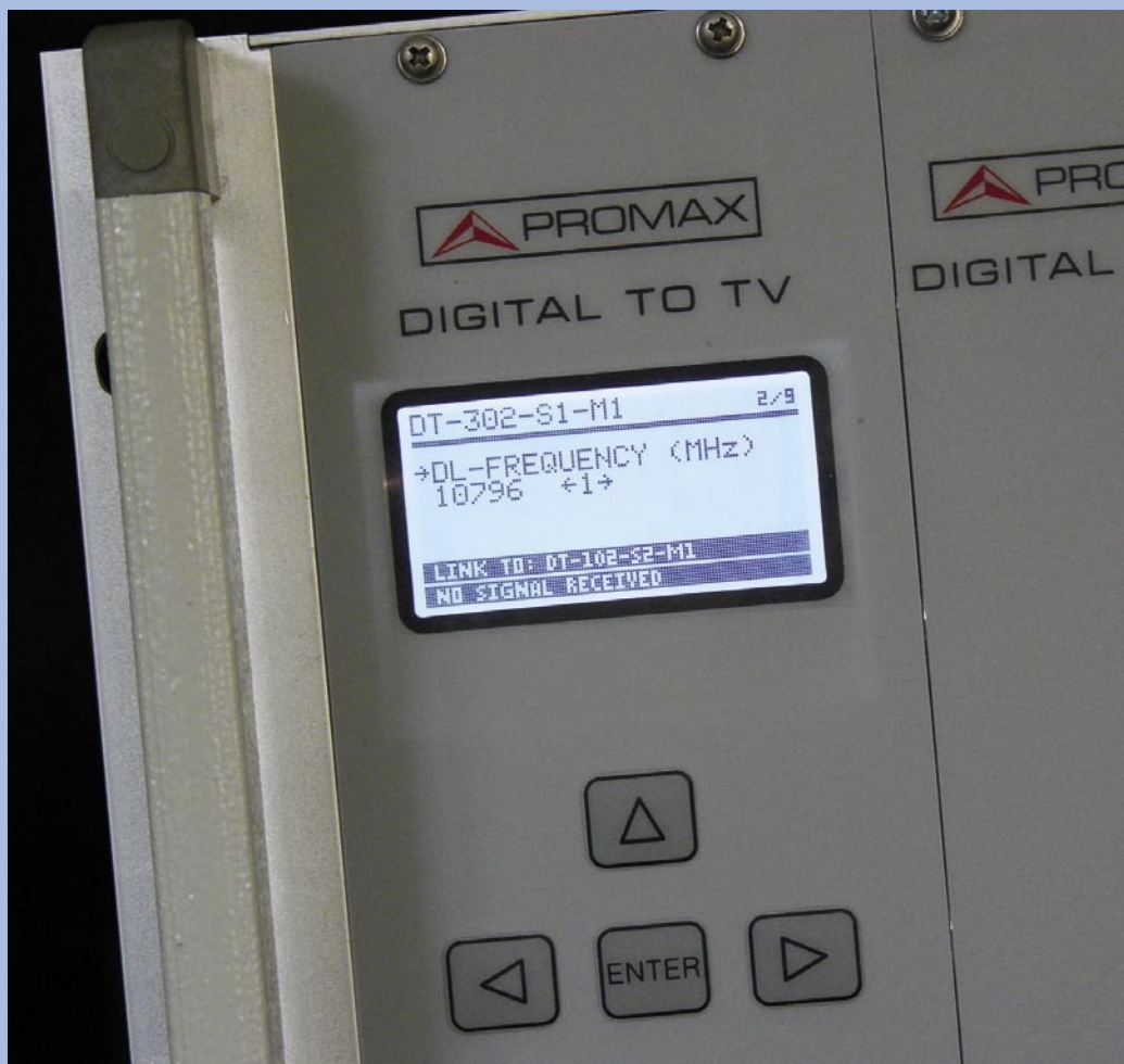
■ Setting up DT 302 module. You can see setting the frequency of the transponder to be received and demodulated to the pure transport stream.
