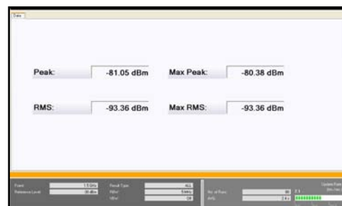
True RMS analysis by selecting Fcent and RBW (Screen NRA Demo Software)
