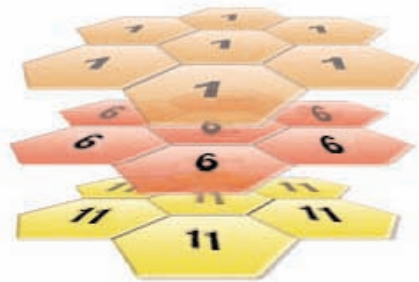
Figure 3: Belden® Wireless Solution Architecture
